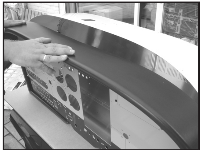
36. While sliding the glaesshield with the lower part over the cabinet, hold it as in the picture above.
