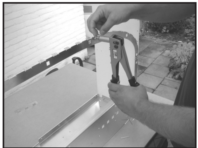
18. Be carefull when mounting all brackets together and check if the mounted brackets form a fluent line.
