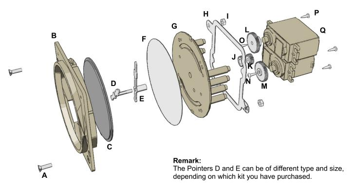
**Remark:** When constructing a single pointer instrument, cut off the lower pointer from the shaft and use the shaft as bearing for the upper pointer. Always mount both gear wheels, even when only one pointer is used.
