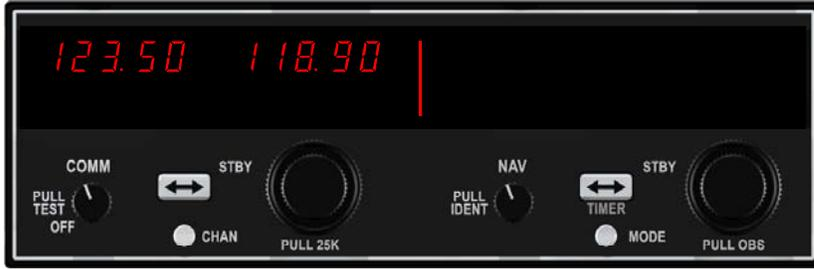
Figure 5. Frequency entered in standby display
