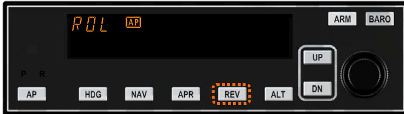
**Figure 21. Back Course Mode using DG from ROL Mode**
