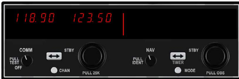
Figure 6, Active/standby frequencies toggle
