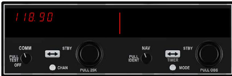
Figure 7. Frequency entered in active entry mode
