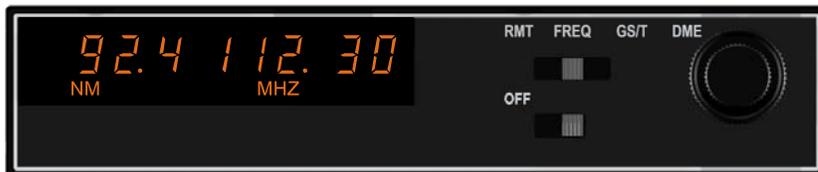
Figure 9. Distance/Frequency FREQ Mode
