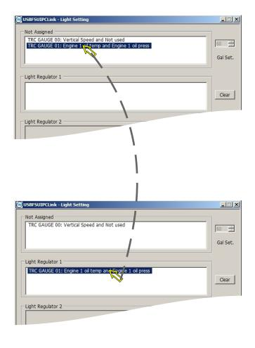
When the USBFSUIPCLink software or the USBFSXLink software recognizes a USB Light Controller, the corresponding window will open and a gauge can be "dragged" from the **Not Assigned** window to an opened **Light Control** window.
