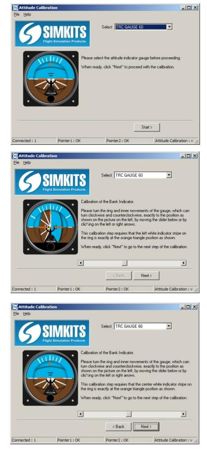
Start the program **"trc\_attitude\_calibration.exe"** and connect the Attitude Indicator to a free USB connector on your PC.
