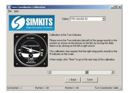
This is the final step to calibrate the Turn & Bank Indicator.
