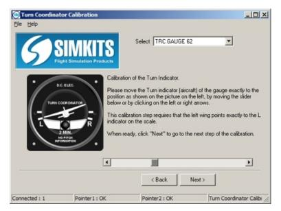
Now the little aircraft which shows the turn position of the plane has to be calibrated.
