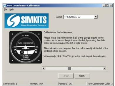
First the little bal (inclinometer or slip-indicator) has to be calibrated.
