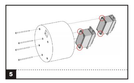
**5.** Remove 2 screws of each servo as shown in the illustration. Position the servos inside the lower part of the housing as shown and mount the servos carefully with the loosened screw.
