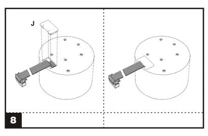
**8.** Move the ribbon cable through the hole in the housing and place the strain relief such a way that the ribbon cable is mounted properly between the space of the strain relief and the housing.
