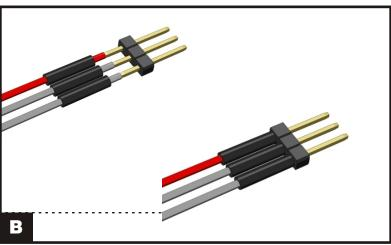
**B:** Separate on one end of the ribbon cable the leads for approx. 3 cm. (approx. 1.2") from each other. Remove the insulation from the end of the ribbon cable for approx. 5 mm. (approx. 0.5").
