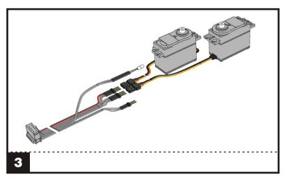
**3.** Connect both servos to the ribbon cable as in the picture. Be sure of the correct polarity. The black wire of the servos must go to the first (red) wire of the ribbon cable and the 4th wire of the ribbon cable.
