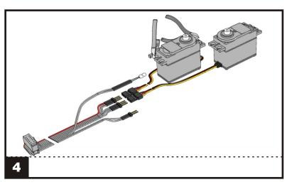
**4.** Now cut mounting the ears from the servo as shown in the illustration.
