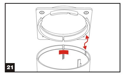
**21.** Mount the front ring onto the housing. Check for the positioning pins and be careful during this mounting not to move the lamp in a wrong position.
