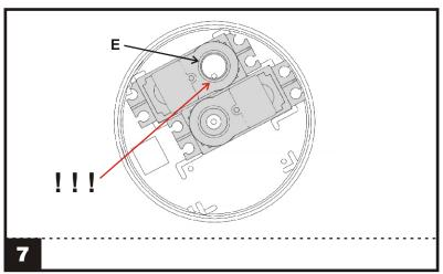
7. Check for the proper position of the servo in the housing. The servo with the cut off ears must be mounted to the side of the housing.
