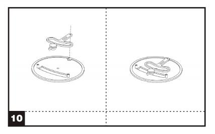
**10.** Position the pendulum on the little plastic shaft on the back side of the front plate as show.
