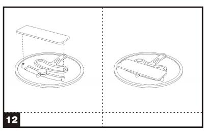
**12.** Now position the small square plate with the two pins on the bushes of the front plate.
