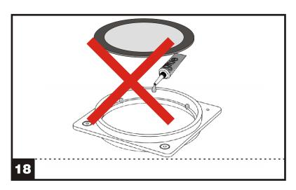
**18/19.** Positioning and gluing the optics on its place has to be done very careful.
