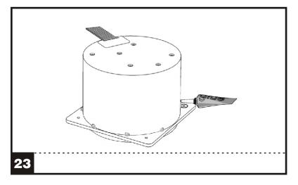
**23.** Finally mount the front ring onto the housing using tiny drops of glue. It is recommended to use about 8 drops around the housing.
