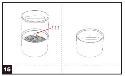
**15.** Mount carefully the front plate with pendulum in such a way on the housing that the small pin of the excentric is positioned exactly. The front plate can only be positioned on the housing one way due to positioning pins.
