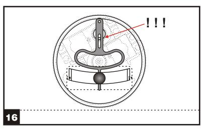
**16.** This drawing shows exactly how the pendulum must be positioned during the construction.
