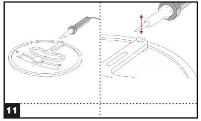
11. Now take a soldering iron and push (very shortly) with the side of the soldering iron onto the little shaft which holds the pendulum.
