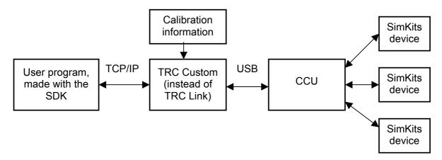
Actual communication between the CCU and the computer is realised via USB.
